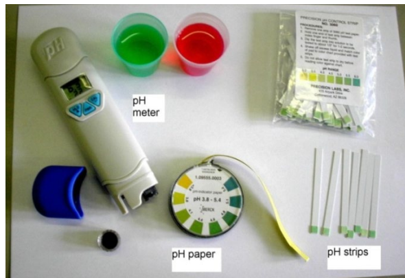
Figure 2. Equipment needed for measuring pH values
