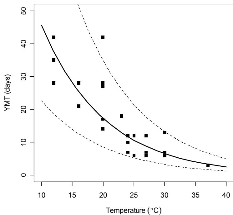
**Figure 2.8** Plot of YMT vs storage temperature. The solid line shows the fitted model with confidence intervals (dashed lines). (Thomas *et al.*, 2006).
