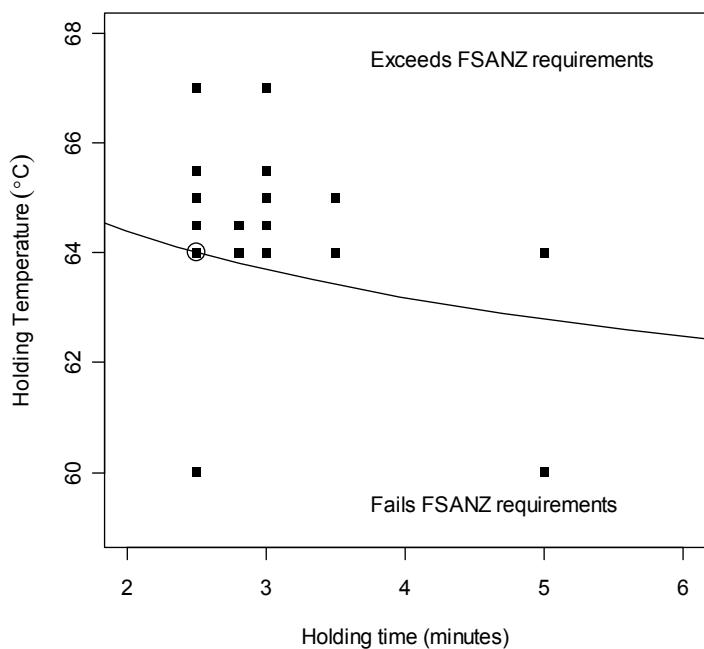
**Figure 2.9** Comparison of reported industry holding conditions (squares) for the pasteurisation of whole egg pulp. The circle represents FSANZ processing requirements. The solid line shows temperature and holding times of equivalent severity ( $z = 4^{\circ}\text{C}$ ) to the FSANZ standard. Combinations of holding times and temperatures to the bottom of the solid line represent under-processing (Thomas *et al.*, 2006).
