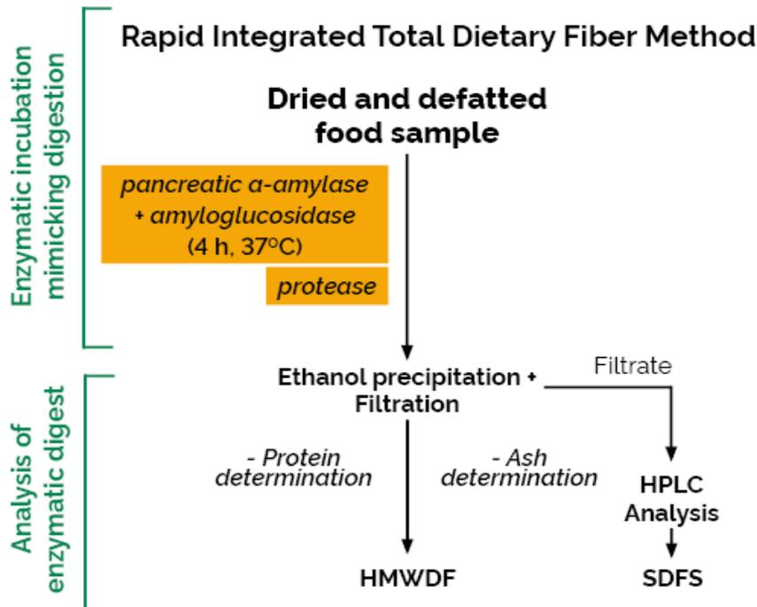
Figure 2. Simplified analytical steps for AOAC 2017.16<sup>3</sup>.
