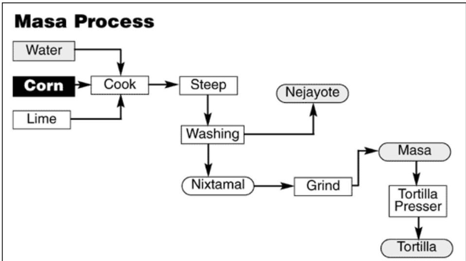
Figure 2: The main corn refining processes and products (Iowacorn<sup>4</sup>)
