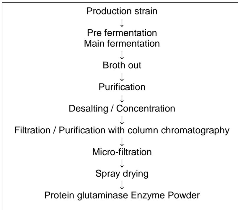
**Fig 3:** Manufacturing Process for Protein glutaminase
